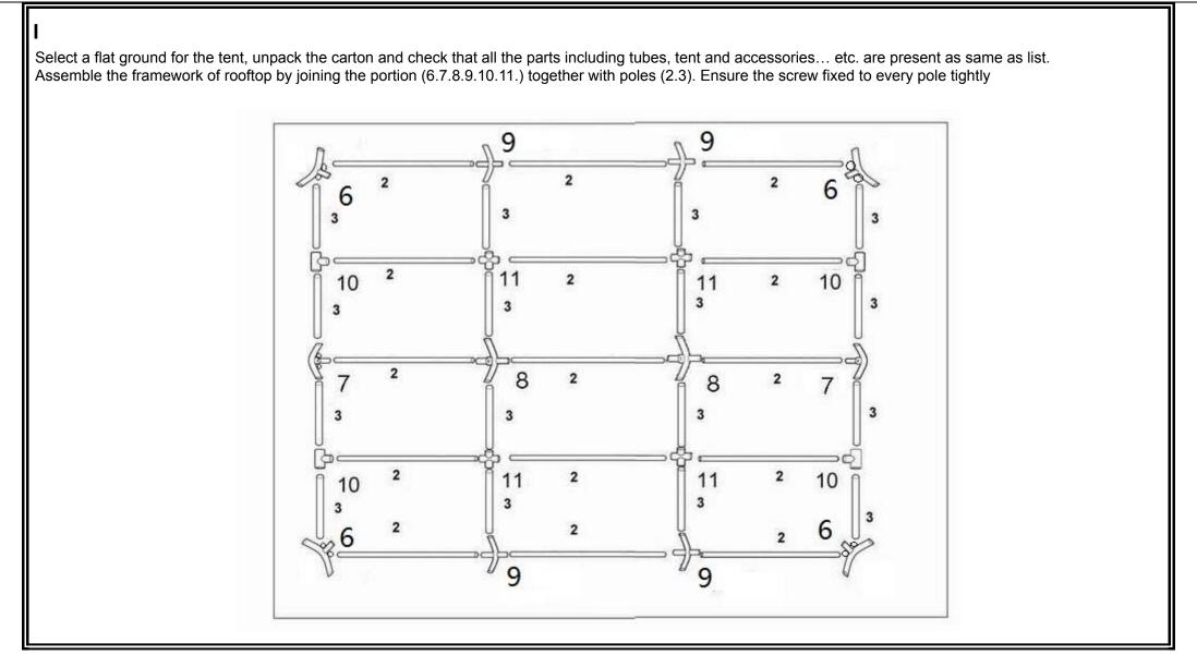
Attach one end of supported pole (4.5) to the joints (7.8) ,Strengthen the frame by using screws and turnbuckle set (17 .) .Long screws are used on all connection between 50mm and 54mm pipe .Short screw are used on connection between 42mm and 38mm pipes .
