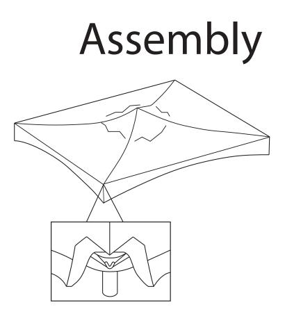
**Step 5**: Assembly the roof cover, pull the corner with handle.
