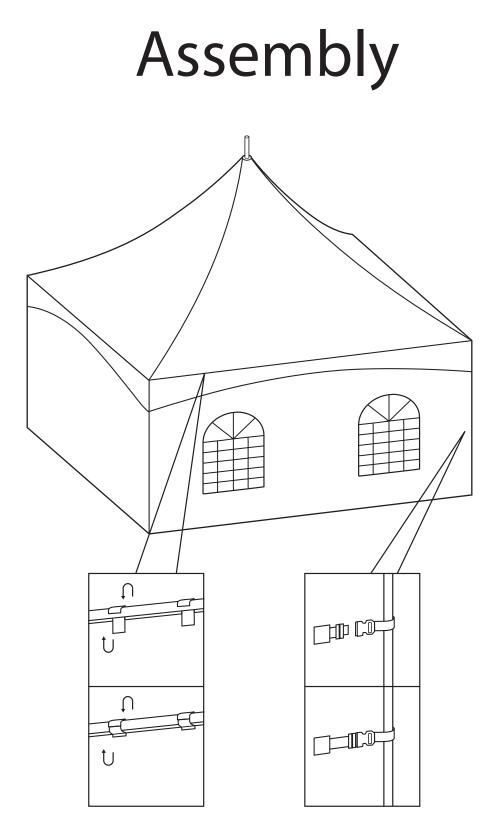
**Step 8**: Suspend all the sidewalls. **Note: use the buckles fix the sidewall on the frame**
