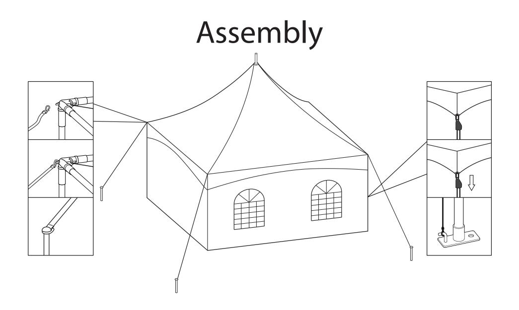
**Step 9**: Fasten the roof tensioning ropes and use the roof tensioning strapes make the tent more stable.
