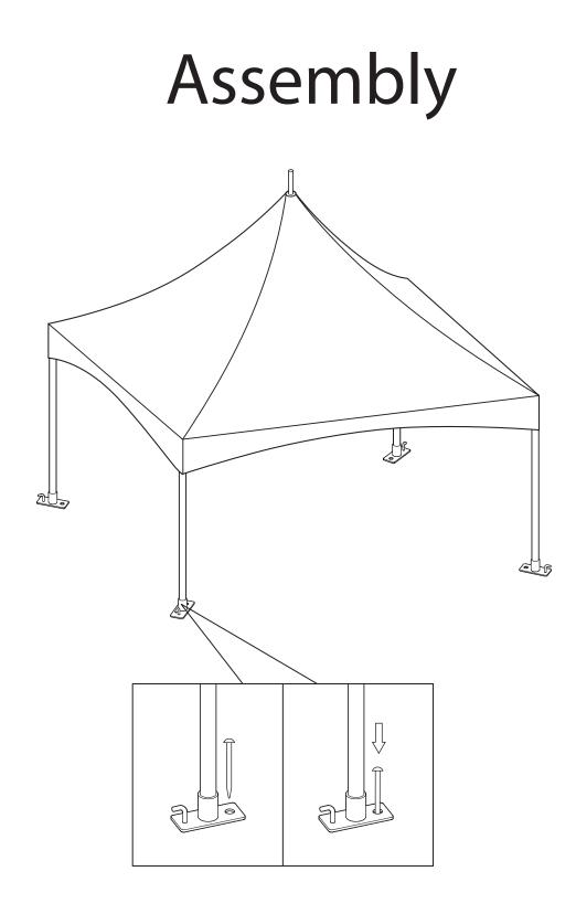
**Step 7**: Insert all the legs to make the tent stand up. **Note: use pegs to fix the tent on the ground**
