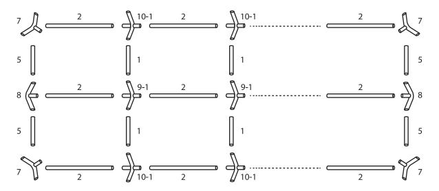
To ensure the screw fixed to every pole tightly. And then use the turnbuckle set which is diagonally across through each section as below.
